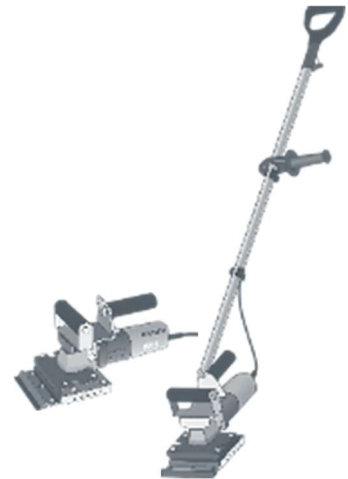
Tools for stripping the existing floor covering (Duro-Stripper, Primo-Stripper)
