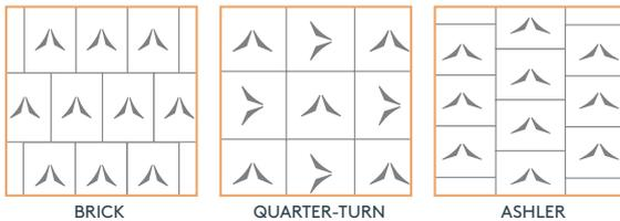
Installation of Carpet Tiles — Directional vs Quarter Turn, some patterns allow the carpet tiles to be laid either using a Directional method or by Quarter Turn method. Other patterns is such that they can only be laid "Quarter Turn" or in a "Random" manner. More information may be found on the relevant product data sheet on our website [www.advanceflooring.co.nz](http://www.advanceflooring.co.nz) or you can call us for further clarification if required.
