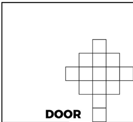
Make sure that no pile material is trapped between the tiles. This central point is a starting point for the gradual placement of the other pieces. It is necessary to apply good pressure when butting the tiles together for a neat fit.
