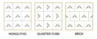
Installation of Carpet Tiles — Directional vs Quarter Turn, some patterns allow the carpet tiles to be laid either using a Directional method or by Quarter Turn method. Other patterns is such that they can only be laid "Quarter Turn" or in a "Random" manner. More information may be found on the relevant product data sheet on our website <u>www.advanceflooringsystems.com</u> or you can call us for further clarification if required.
