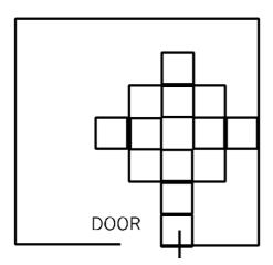
Make sure that no pile material is trapped between the tiles. This central point is a starting point for the gradual placement of the other pieces. It is necessary to apply good pressure when butting the tiles together for a neat fit.
