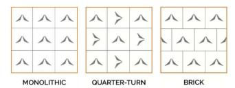
Installation of Carpet Tiles — Directional vs Quarter Turn, some patterns allow the carpet tiles to be laid either using a Directional method or by Quarter Turn method. Other patterns is such that they can only be laid "Quarter Turn" or in a "Random" manner. More information may be found on the relevant product data sheet on our website <a href="https://www.advanceflooringsystems.com">www.advanceflooringsystems.com</a> or you can call us for further clarification if required.
