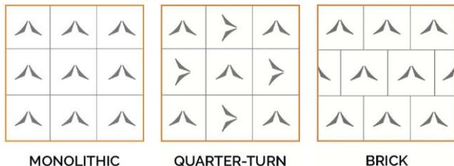
Installation of Carpet Tiles — Directional vs Quarter Turn, some patterns allow the carpet tiles to be laid either using a Directional method or by Quarter Turn method. Other patterns is such that they can only be laid "Quarter Turn" or in a "Random" manner. More information may be found on the relevant product data sheet on our website [www.advanceflooringsystems.com](http://www.advanceflooringsystems.com) or you can call us for further clarification if required.
